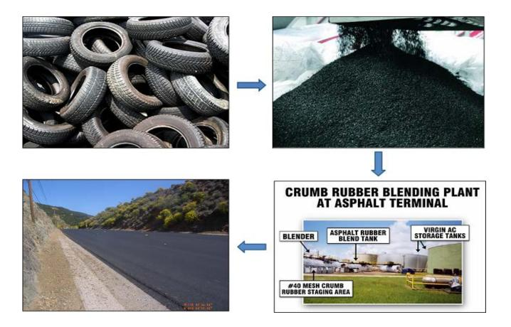
Rubberized asphalt concrete provides a longer lasting, more durable surface course than asphalt paving which doesn't contain crumb rubber. Thus, the frequency of maintenance is greatly reduced due to the longer life cycle. Rubberized Asphalt Hot Mix is a very common product manufactured at most asphalt plants.
