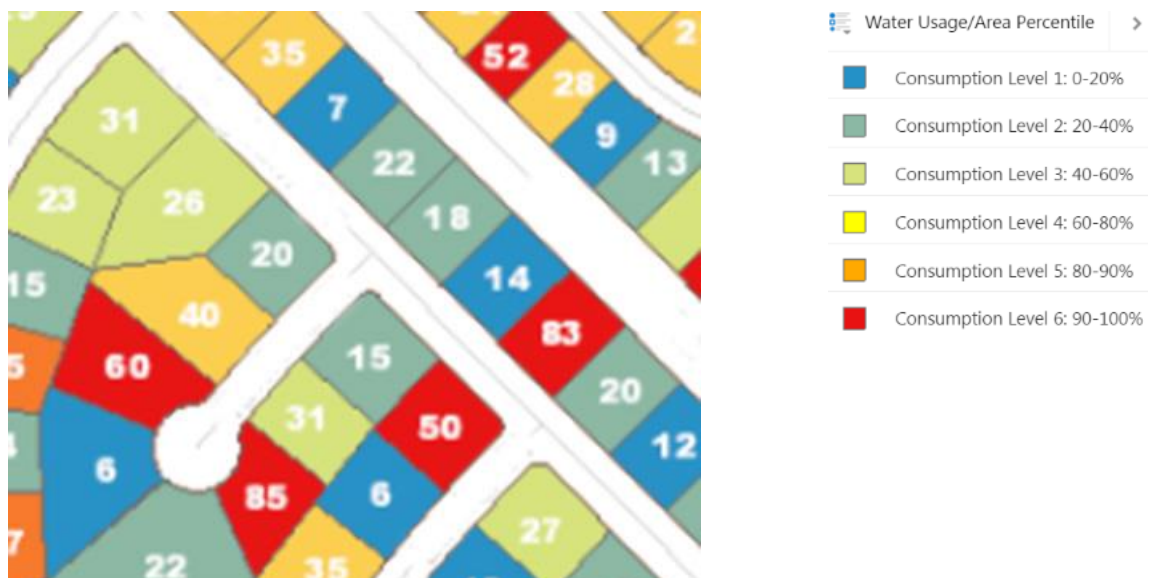
Figure WU-4: Water use for a single-family home neighborhood. Colors indicate the percentile classification of each parcel. Data labels represent the previous 2-month total usage in HCF. The usage disparity between similar sized parcels is striking.
